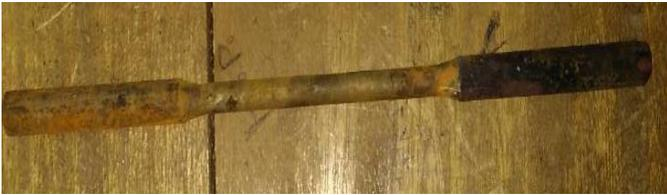
Figure 4: Specimen after quenching
